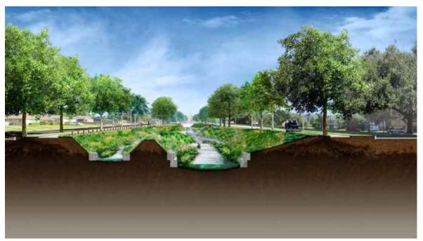
Neutral grounds designed to recharge aquifer, mitigate the rate of subsidence
