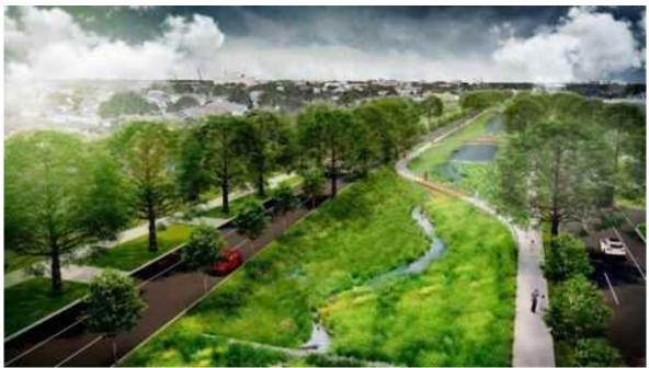
Neutral grounds designed as extension of flood control pump station wet wells
