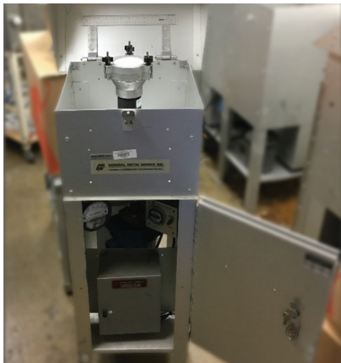
PS-1 high-volume air sampler with media installed
