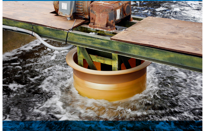
"Paint Wheel" rotating at 16 knots during dynamic test of hull coatings for ASTM D4939
