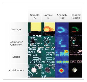
Table showing example anomalies detected by RAICS with the general anomaly category along the left and the data type above.
