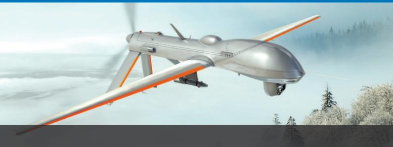
HeatCoat™ Active, In-Flight Ice Protection System
