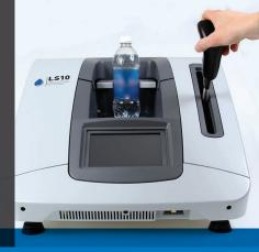
The LS10<sup>™</sup> is a bottle liquid scanner that distinguishes threat liquids, aerosols, and gels (LAGs) from benign substances and alerts security personnel to suspicious contents quickly and accurately.
